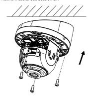
Figure 2-24 Fix the Camera to Wall Mounting Bracket
