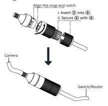
Figure 2-27 Water-proof Accessory Installation
