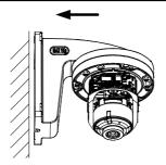
Figure 2-12 Fix the Wall Mounting Bracket to Wall
