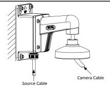
Figure 2-16 Cable Routing
