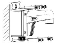
Figure 2-14 Fix the Bracket
