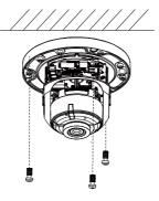
Figure 2-5 Fix the Mounting Base
