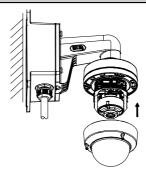
Figure 2-18 Install the Bubble
