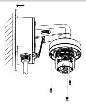
Figure 2-17 Fix the Camera to Wall Mounting Bracket
