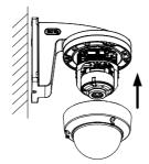
Figure 2-13 Install the Bubble
