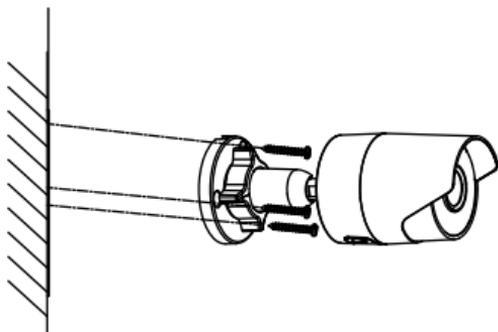
Figure 2-4 Secure the Camera to the Ceiling
