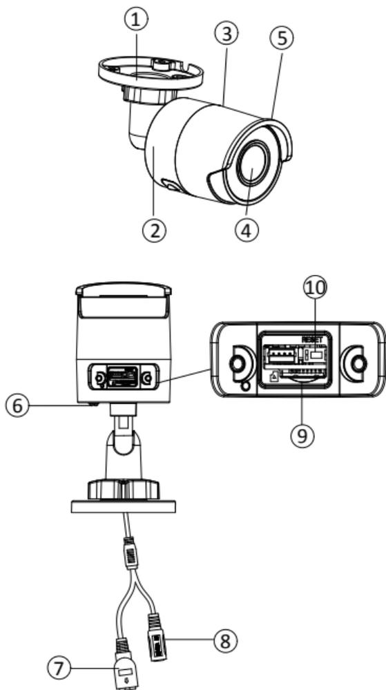
Figure 1-5 Type III Bullet Camera
