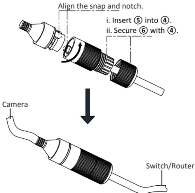
Figure 2-7 Water-proof Accessory Installation
