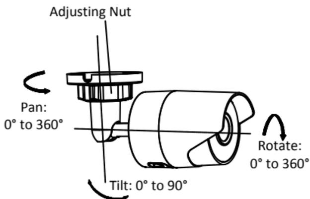
Figure 2-5 3-axis Adjustment
