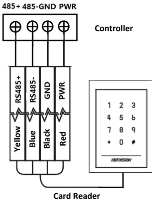
Figure 3-4 Wiring for RS-485 Communication Mode
