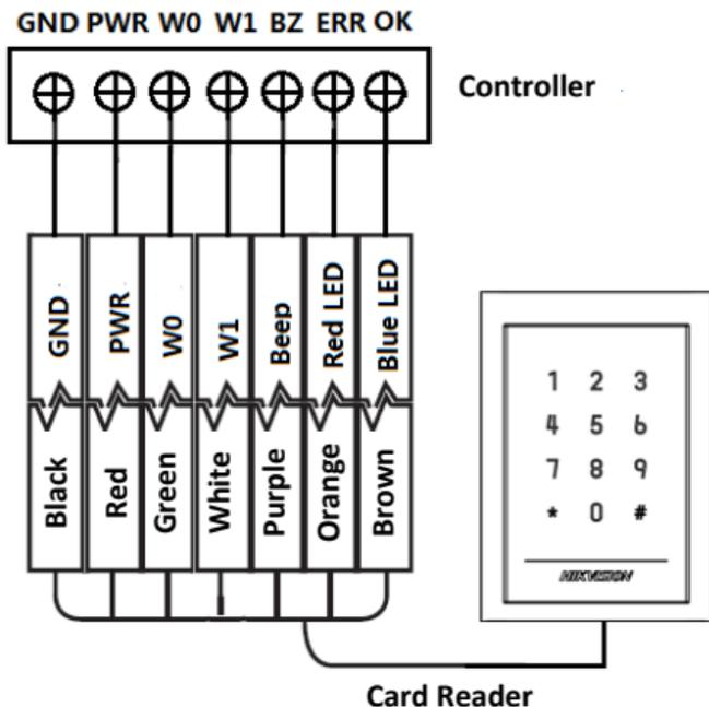
Figure 3-5 Wiring for Wiegand Communication Mode
